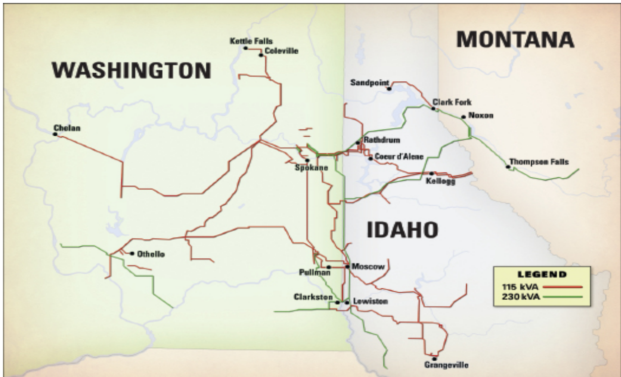
Figure 5.1: Avista transmission system
